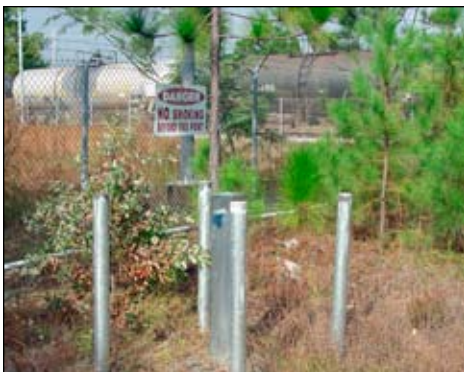
A monitoring well at Simmons Army Airfield's former fuel point hints at the environmental damage caused by several above- and below-ground fuel releases. Monitoring activities identified a major plume of free product below the tank area and the contamination is being actively addressed via vacuum-enhanced free product recovery. Since February 2008, almost 200 of the estimated 250 gallons of free product recoverable has been removed from the ground.
