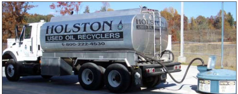
Petroleum product recycling is accomplished with help from an outside recycling plant. The contractor pumps used vehicle motor-oil through a high-velocity recovery pump, returns the oil to a central facility for filtering processes with diesel fuel, and re-injects the fuel/oil mixture back into the retail system for use as residential and industrial heating oils, allowing for greater used oil reuse. The NCARNG no longer has to transport, store, or otherwise dispose of used oil products or purchase greater quantities of diesel fuel.
