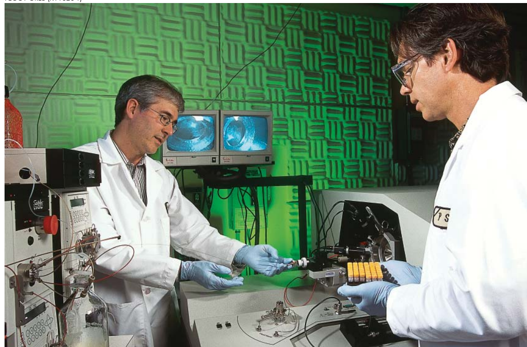
Chemist Chris Silva (left) and research leader J. Mark Carter load samples for analysis via nanospray liquid chromatography coupled to mass spectroscopy. This state-of-the-art technology characterizes BSE prions with unprecedented precision.
