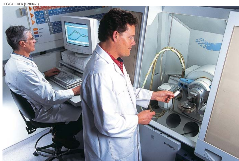
Chemists Greg Gray (left) and William Orts use x-ray diffraction to characterize agricultural fibers for use in biobased products.
