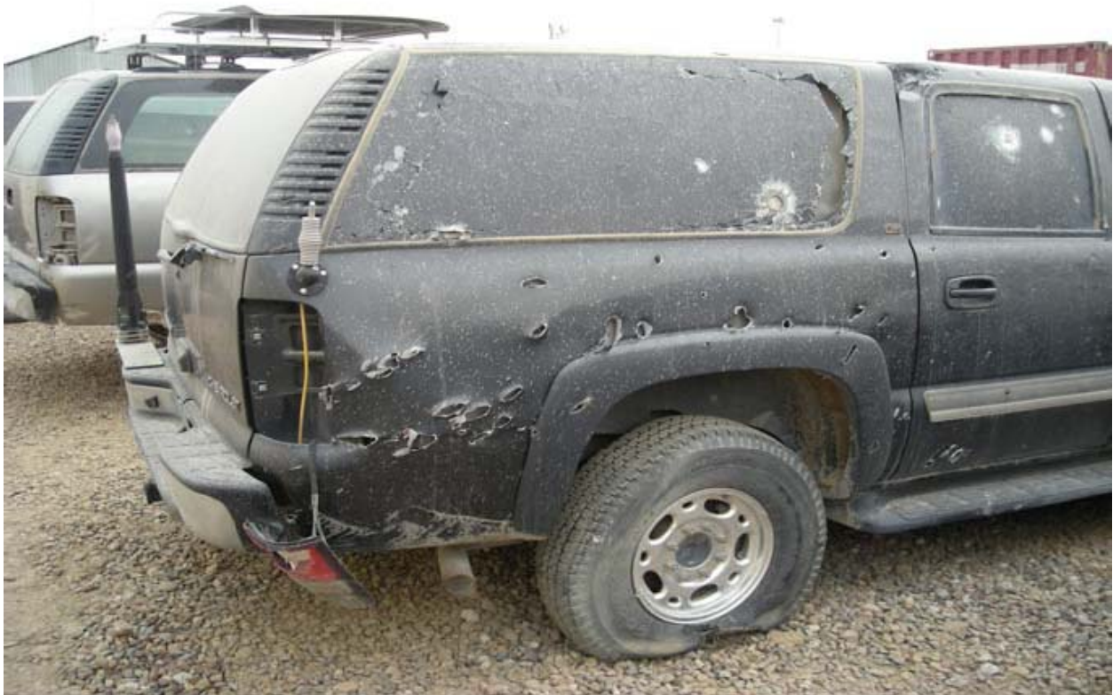
Photograph of a USAID/Iraq armored vehicle with shrapnel damage in Basrah, Iraq, in March 2008. Source: OIG/Iraq
