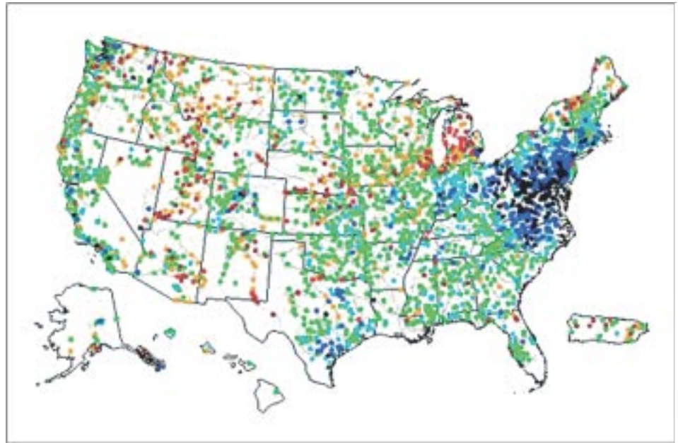
Fig. 2. This WaterWatch real-time map shows flow conditions at USGS stream gauging stations. Darker dots are gauges recording high flows. The map is for the day following the passage of Hurricane Isabel on the east coast (19 September 2003, 16:20 ET). The colors represent percentiles of stream flow that are calculated from historical observations for the current day of the year at stream gauging stations with at least 30 years of record. A major attribute of WaterWatch is a point-and-click feature that allows users to retrieve maps and graphs of real-time river stage and discharge data for individual stations. It includes pages that summarize real-time stream flow, daily stream flow, 7-day average stream flow, flood and drought flows, and graphs of recent conditions. Water-Watch also serves as a geospatial front-end to the new USGS online National Water Information System ( http://water.usgs.gov/nwis ), which provides open access to real-time and historical surface water, groundwater, and water quality data. NWIS-Web contains over 181 million historical daily stream flow values and makes them available in graphical or tabular form. These new data delivery systems greatly simplify the process of obtaining stream flow data from the USGS.
