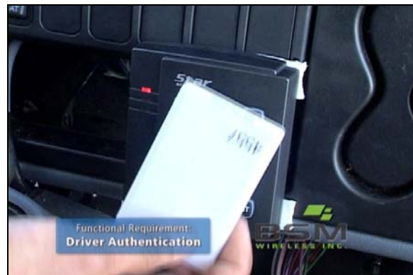
Figure 10. BSM Wireless Driver Authentication Stage 1: Proximity Card
