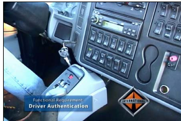
Figure 14. International Truck and Engine Driver Authentication Keypad Code Entry
