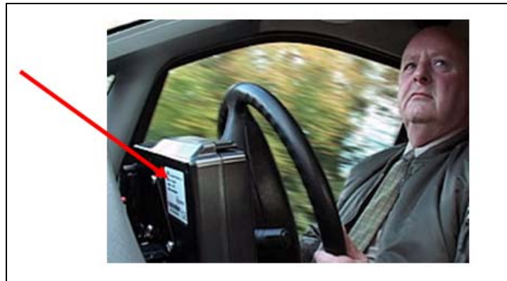
Figure 45. Truck Cab Outfitted With Swipe Card System.
