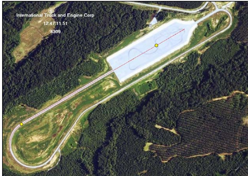
Figure 31. International Truck and Engine VST Demonstration Test at Arterial Speed Vehicle Trajectory Immediately before Stopping (Run 1)
