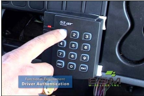
Figure 11. BSM Wireless Driver Authentication Stage 2: Keypad Code Entry
