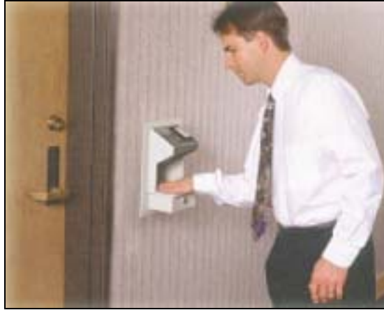
Figure 58. Hand Geometry Measurement System in Use.
