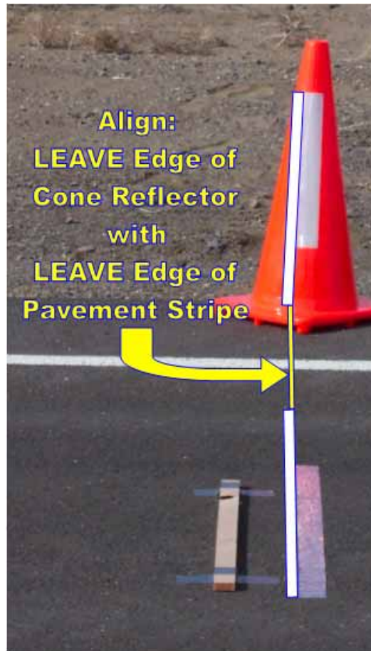
Figure 84. Photo. Placement of vertical photocell target in relation to section starting location.
