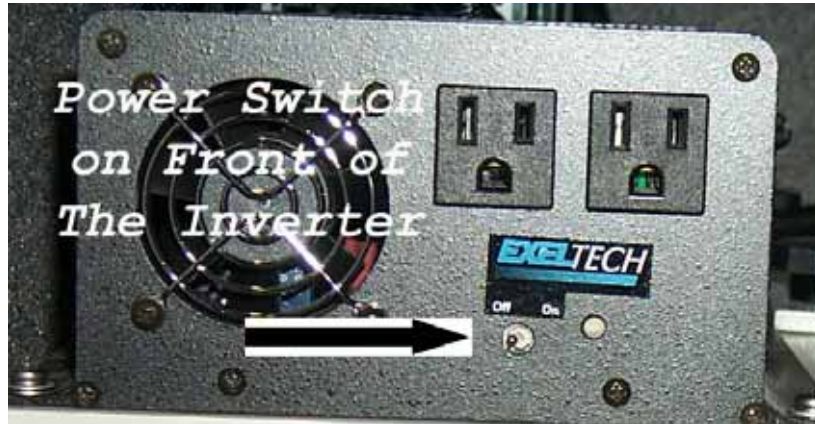
Figure 8. Photo. Inverter switch.
