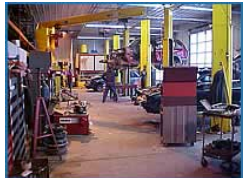
Incoming vehicles should be inspected, drained and dismantled in one area, on an impervious surface such as a concrete pad, and under a cover or roof. (Photo courtesy of NH DES, from EPA Region 1)
