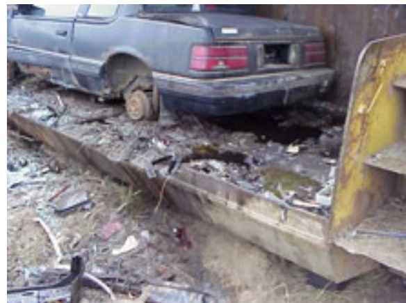
Toxic fluids leaking from this crusher are a violation of the Clean Water Act. (EPA Region 9 photo.)
