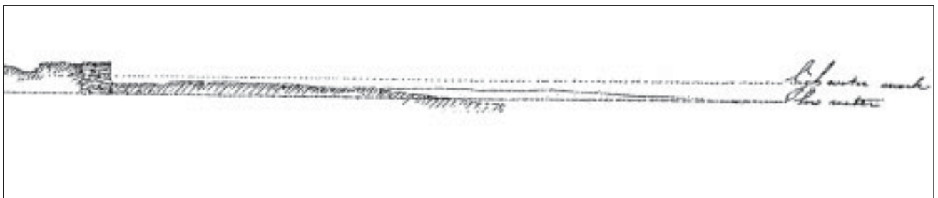
Figure 2.2. Detail of 1819 plan by Captain William Tell Poussin entitled "Reconnoitering of Chesapeake Bay, State of Maryland; Plan and Profiles of Fort McHenry," showing profile of seawall and mudflats at low and high tide marks. National Archives II, College Park MD. Record Group 77.
