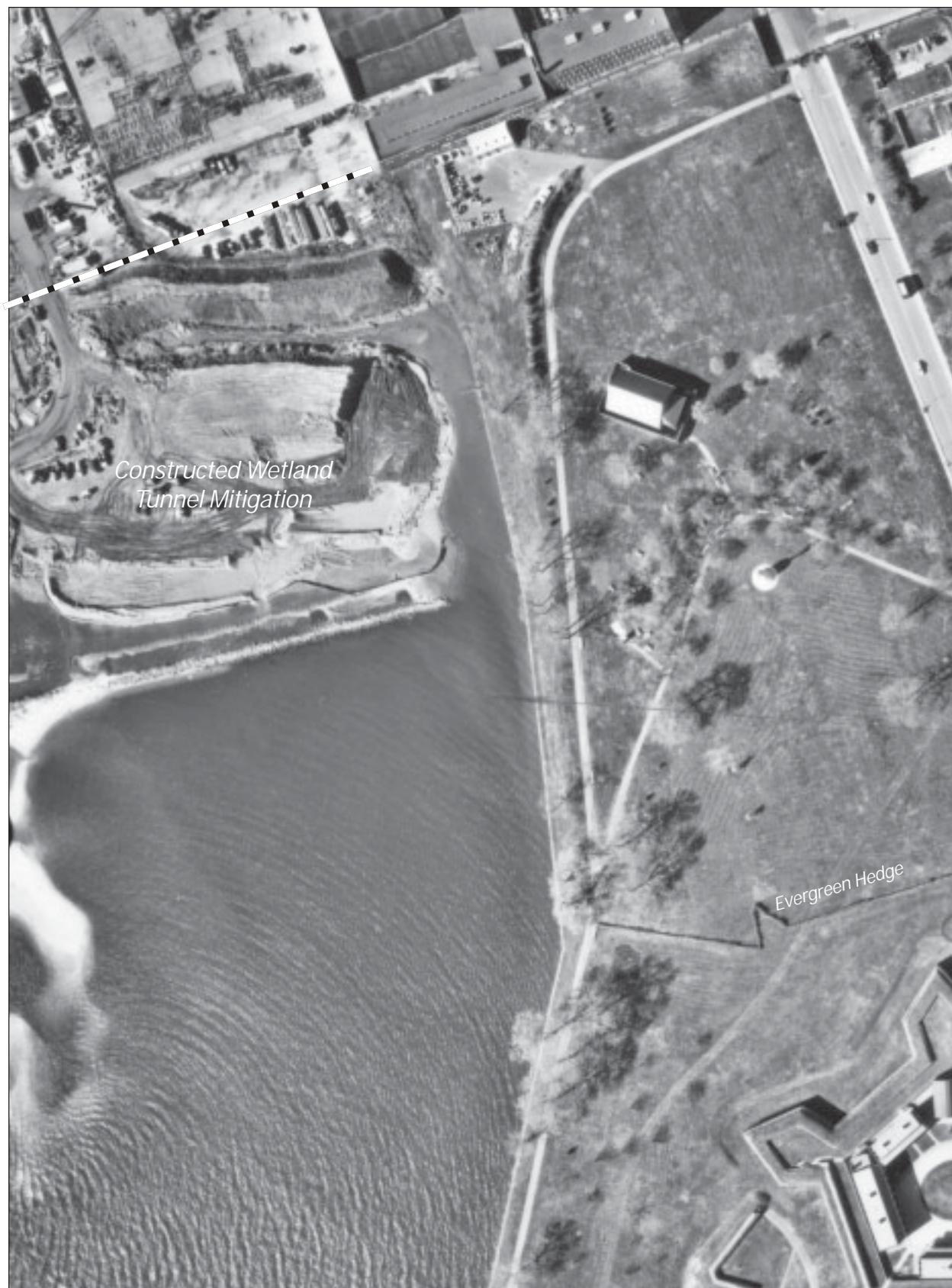
Figure 5.29. Aerial photograph, 21 November 1983. This image shows the area of artificial constructed wetland, built as environmental mitigation for the Fort McHenry tunnel project. Fort McHenry Library Special Collections.
