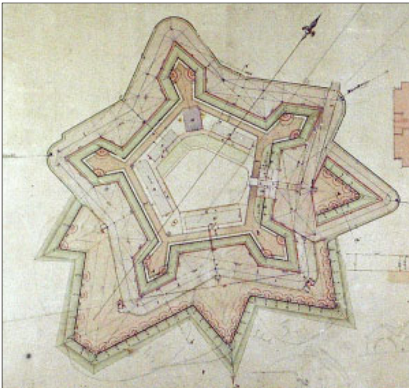
Figure 2.4. Detail of 1840 plan by Capt. Fred A. Smith entitled "[Plan of] Fort McHenry, Baltimore, from dimensions furnished by Capt. Henry A. Thompson," showing alterations to the Star Fort including the new water battery and the remodeled entrance to the sally port. National Archives II, College Park MD. Record Group 77.
