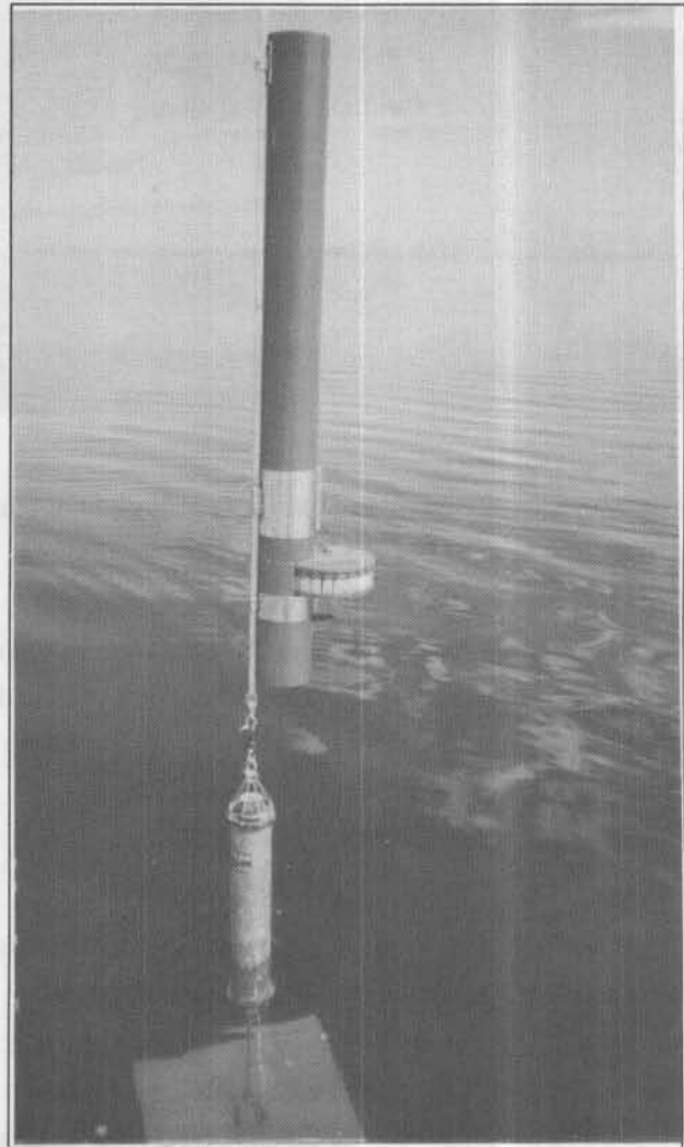
Figure 18. The GLERL-designed sequential sediment trap ready for deployment in Lake Michigan.
