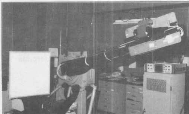
Figure 20. Barium sulfate panel mounted on five-axis positioner. The rotating boom, on which the detector is mounted, is shown at an angle approximately +20^\circ from normal to the panel.
