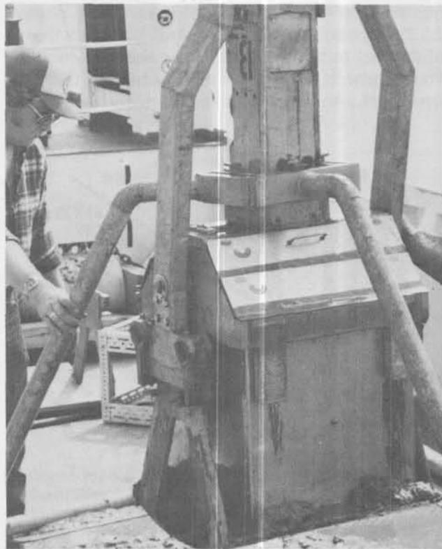
Box corer used to collect sediments from the Canadian survey ship Limnos . As part of a cooperative study between the Canada Centre for Inland Waters and GLERL, sediments are being collected from each of the Great Lakes.
