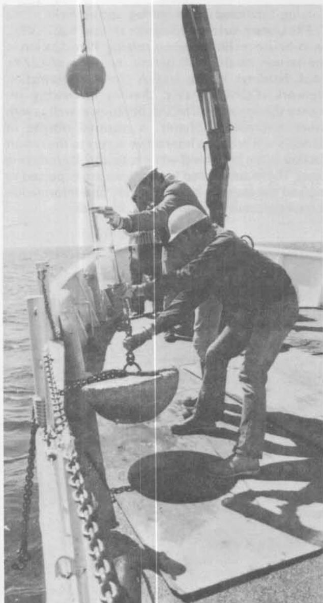
Crew of the research vessel Shenon recovering a sediment trap mooring from Lake Michigan. Deployment and retrieval of the instruments used to collect basic data are important functions requiring a well-equipped boat.
