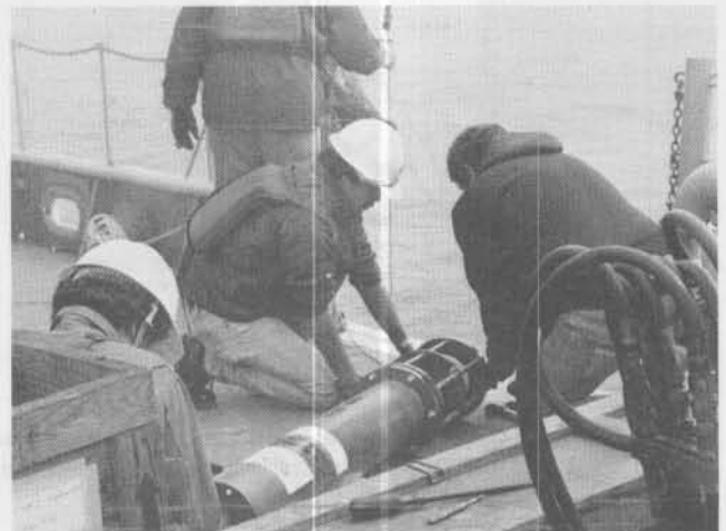
Deployment of a current meter in Lake Michigan. These meters record currents and temperatures for 1 year and provide the fixed array data used in water movement studies.
