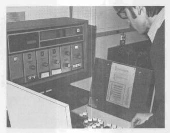
Scientists using the liquid scintillation counter in the GLERL biology laboratory.
