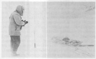
GLERL technician preparing to collect data on radiation transmittance through ice in the photosynthetically active range.
