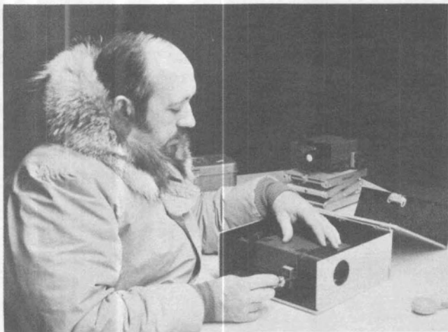
Scientist calibrating a radiometer in the ice laboratory. More accurate readings are obtained when the instrument has been calibrated in a temperature environment close to that in which it will be used. This workroom is kept at +20^{\circ}\text{F} .
