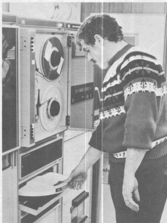
Computer specialist loading a disc pack into the Hewlett-Packard 9603A Scientific Measurement and Control System. Measurement tapes taken directly from instruments must be converted from analog to digital, reduced, and edited on this system before they can be analyzed on the CDC 6600 Computer.
