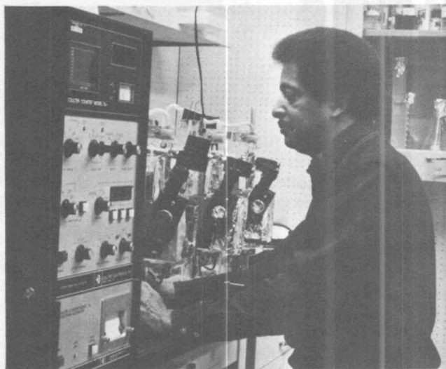
Technician calibrating the Coulter Counter in the biology laboratory. This instrument is being used to count particles in zooplankton grazing experiments.
