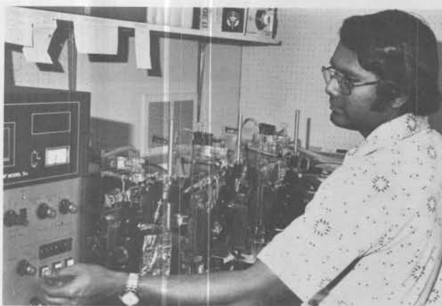
Technician using the Coulter Counter. This is used to determine the particle-size spectrum in lake water. By studying changes in these spectra, GLERL scientists are determining grazing rates on various classes of algae.
