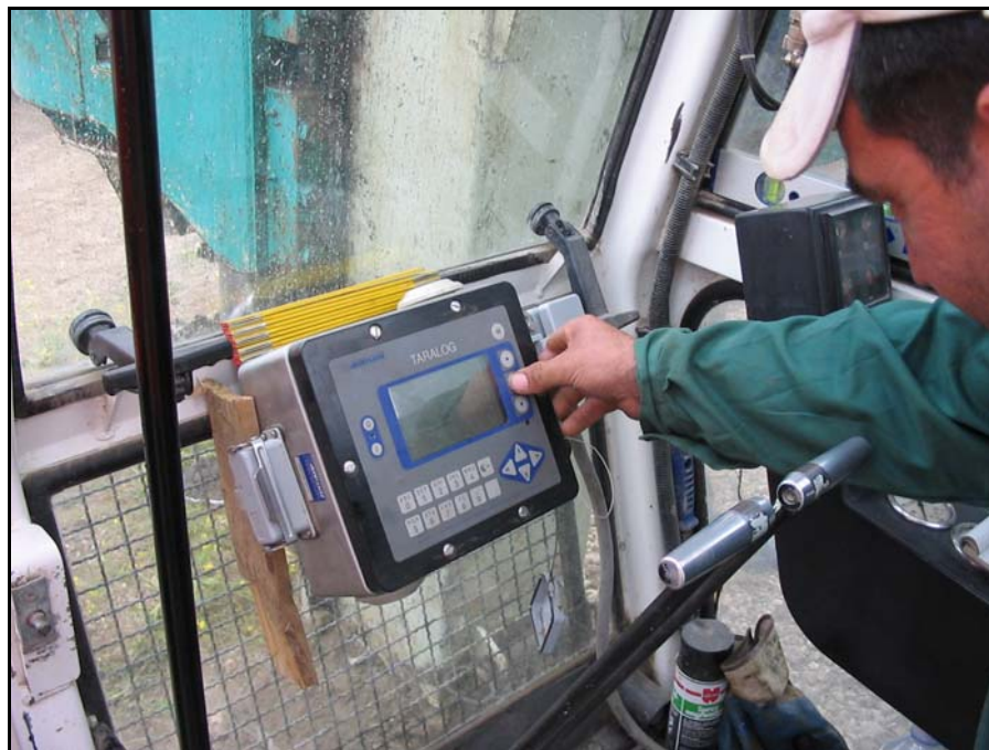
Figure 7.1: Operator with Cab Mounted Display Used to Control Drilling
