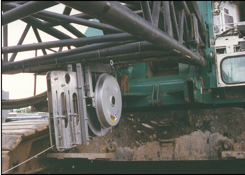
Figure 7.2: Depth Encoder Mounted on Crane Boom
