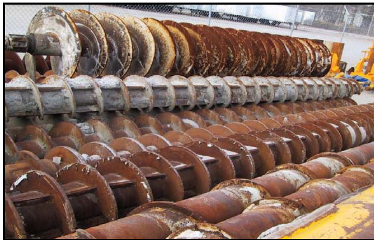
Figure 4.7: Augers for Different Soil Conditions: Auger for CFA Piles in Sandy Soil (Top) and Augers for DD Piles (Bottom)
