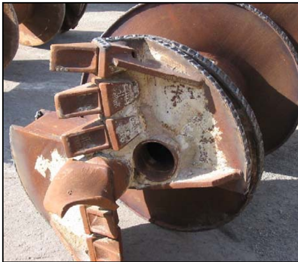
Figure 2.7: Hole at Base of Auger for Concrete
