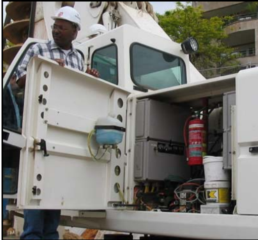
Figure 7.4: Pressure Sensors on Hydraulics to Monitor Rig Forces
