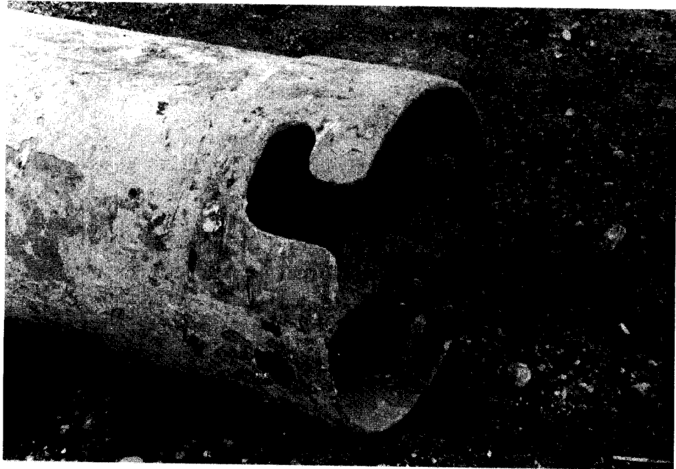
Figure 5.3. J slots in top of casing for use with casing twister (Photograph courtesy of Herzog Foundation Drilling, Inc.)
