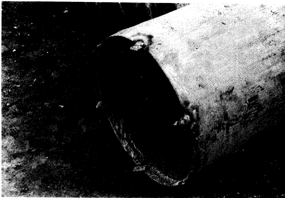
Figure 5.4. Teeth for use in sealing casing into rock (Photograph courtesy of Herzog Foundation Drilling, Inc.)
