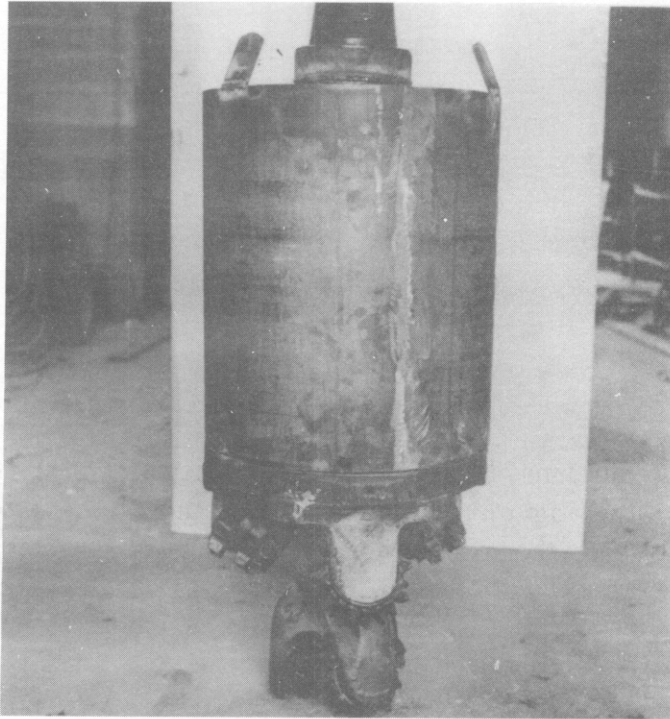
Figure 4.13. Full-faced tool with roller bit (Photograph courtesy of Caissons, Inc.)
