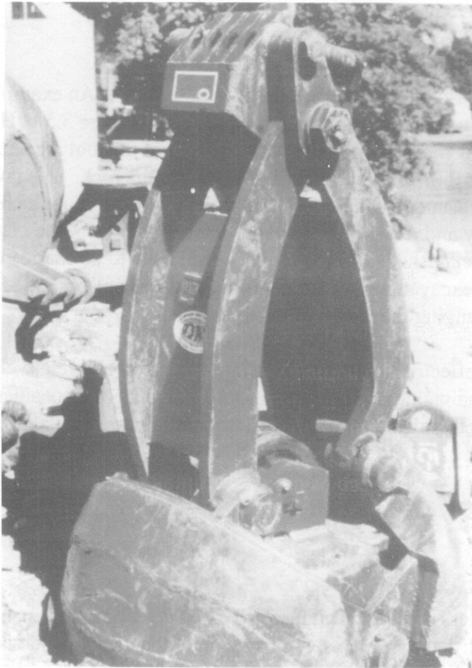
Figure 4.17. A typical grab bucket (Photograph courtesy of John Turner)
