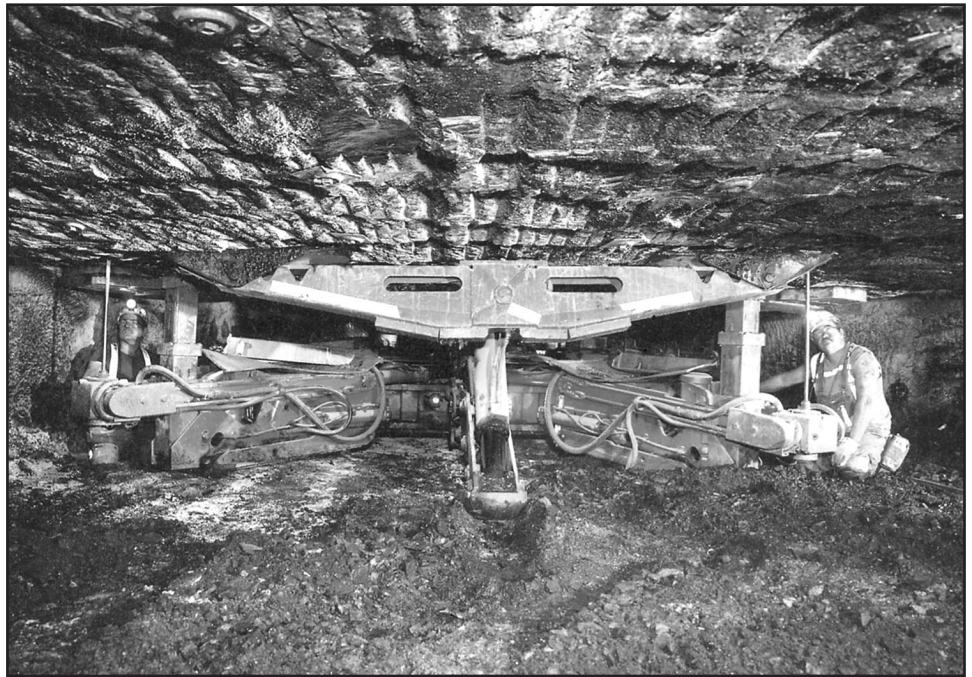
Figure 4: Miners Working in “Low Coal” (a Mine No More Than 40” High)
