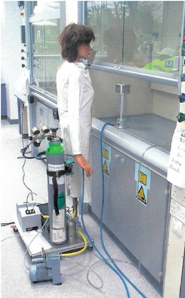
Figure 3. Mannequin simulates worker exposure during a tracer gas test.
