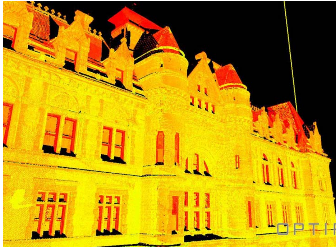
Figure 15: Second example of a registered point cloud - historic building. (Courtesy of Optira)
