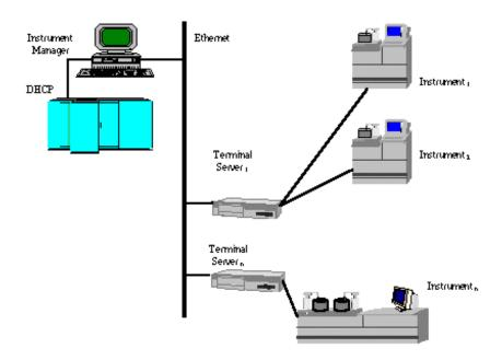
The above example makes use of the Instrument Managers ability to communicate using the DEC LAT network protocol. Instruments are connected to Terminal Servers throughout the institution. The Terminal Servers are attached to the Ethernet network. The Instrument Manager can connect to the individual Terminal Server ports using an Ethernet adapter and the LAT protocol. This allows the Instrument Manager to be placed anywhere in an institution (Lab, IRM, etc.).
