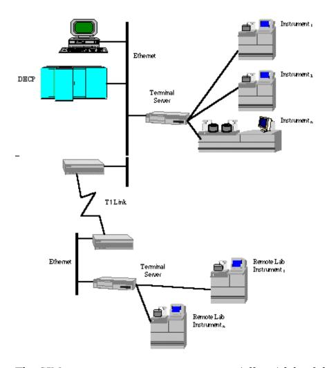
The GIM can access instruments in remote (off-site) labs if the remote sites are connected to the main network. The above example shows the use of a T1 link to create a wide area network (WAN).
