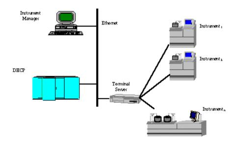
The above example demonstrates the Instrument Manager running two network protocols simultaneously. The DEC LAT protocol is used for communicating with instruments via Terminal Servers. The TCP/IP protocol is used to communicate with the DHCP system. Since TCP/IP can use the Ethernet network, communication speeds between DHCP and GIM are much faster than standard serial communications.
