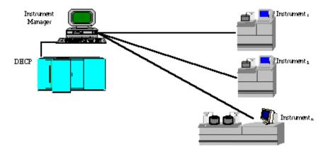
In this configuration, all devices are connected to the Instrument Manager using an Arnet multi-port serial board. A single connection to DHCP assumes the use of the DHCP Laboratory Universal Interface (HL7 protocol). If the Universal Interface is not available, the Instrument Manager can be interfaced to DHCP in Instrument Emulation Mode. The Instrument Manager can be setup to emulate one of the sites existing interfaces. Listed below is an example of instrument emulation:
