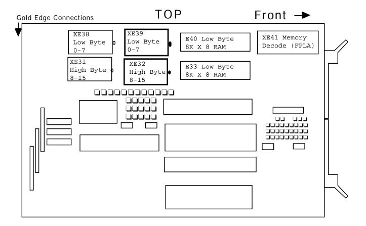
9. Orient the new chips with the chips in XE39 and XE32.
