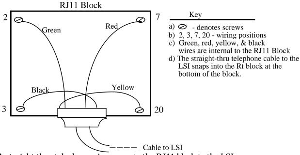
b. A straight thru telephone wire connects the RJ11 block to the LSI.
