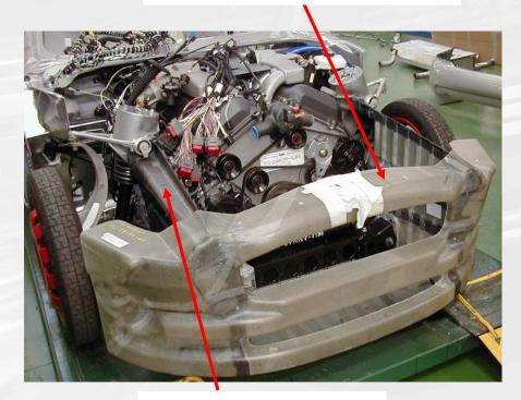
**Cast Aluminum Shock Tower Adhesive Groove Aluminum Tub** (315mm long x 53mm deep) Composite Crash Rail
