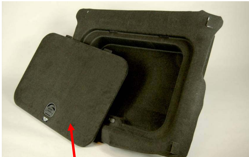
Sandwich panel load floor on the 2006 Ford Escape
