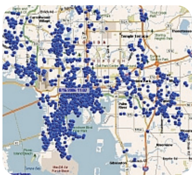
The IntelliOne Roadway Speed Measurement System uses cell phone signals to map roadway speeds for all highways and surface streets where mobile phone coverage exists. The blue dots represent a snapshot of all active mobile phones from a single carrier's network in Tampa, Fla. Credit: IntelliOne Technologies Corporation.
