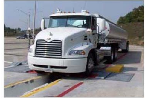
A commercial tanker truck undergoes a Performance-Based Brake Test
