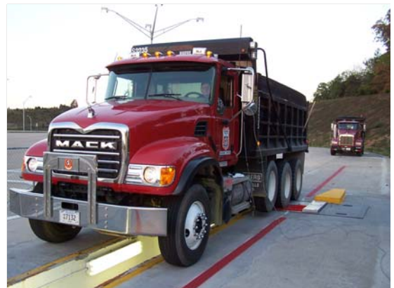
BWPT Vehicle Undergoing a PBBT Test
