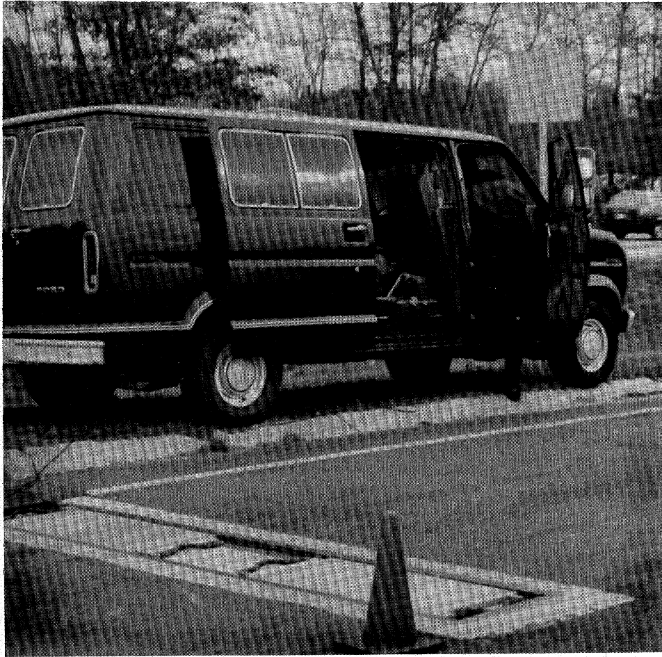
Portable WIM 300 system weighpads installed in roadway cut-out. When not in use dummy grids are installed.
