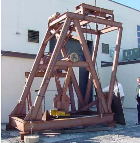
Figure 2 Bulk Fracture Charpy Machine (BFCM) for pendulum impact testing
