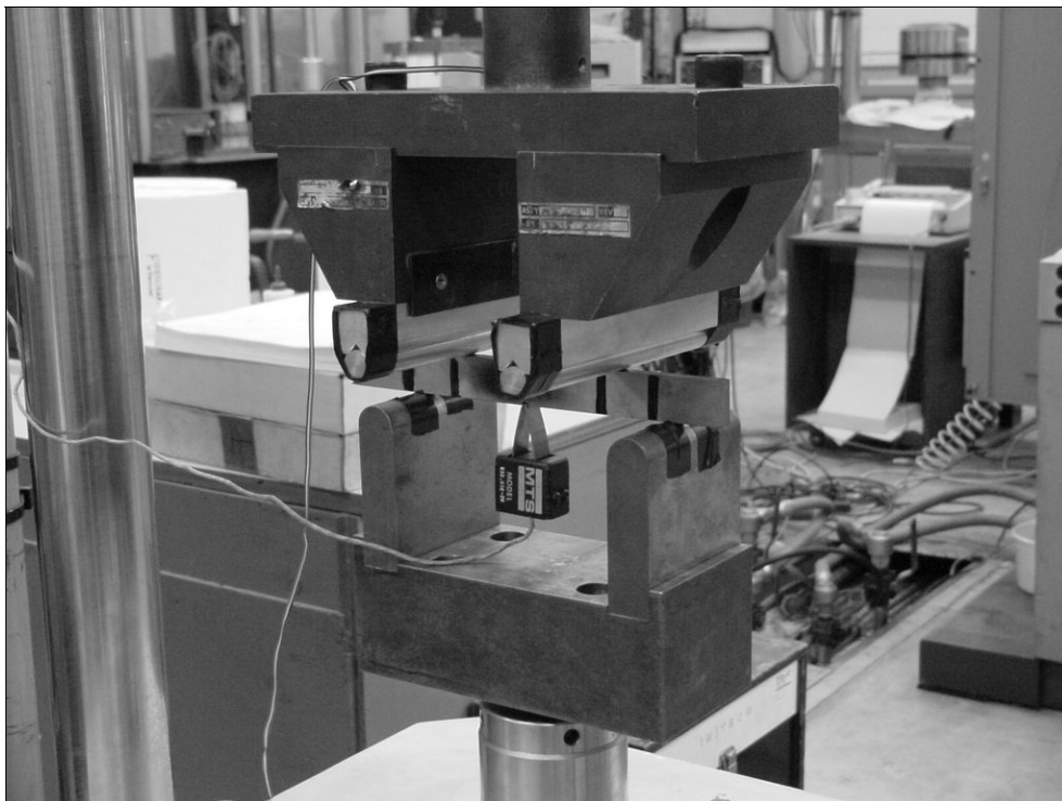
Figure 12. FCG Testing Setup for the SE(B) Specimen Geometry Used in Phase A
