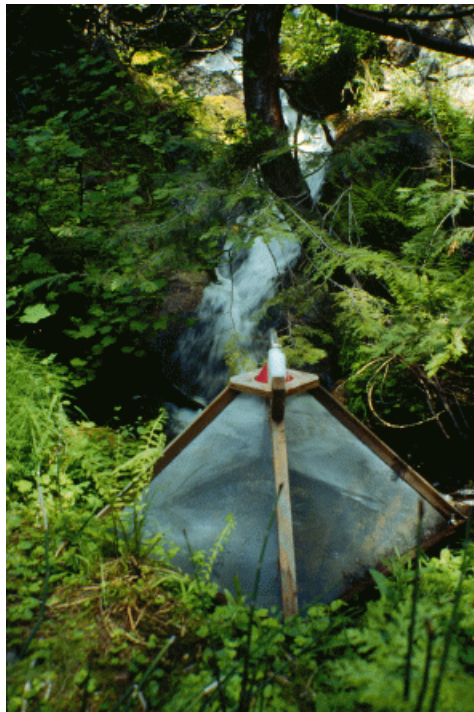
Figure 3.32-1. Pyramidal trap used for sampling macroinvertebrates. Trap is placed within stream.
