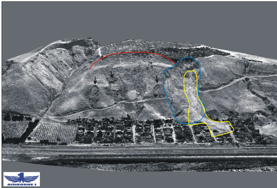
Figure 3b. Oblique LIDAR image of La Conchita after the 2005 landslide. Outline of 1995 (blue) and 2005 (yellow) landslides shown; arrows show examples of other landslides in the area; red line outlines main scarp of an ancient landslide that involved the entire bluff. The deep canyon on the left produced major debris flows in both 1995 and 2005. Image courtesy of Airborne 1 Corporation, El Segundo, Calif.
