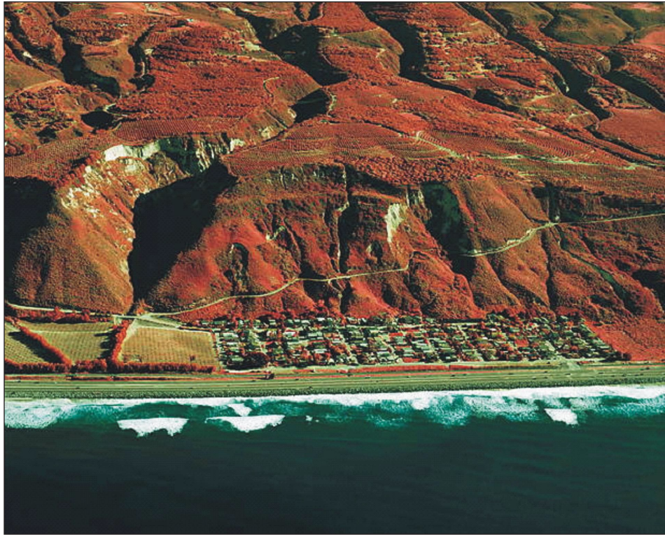
Figure 3a. Oblique false-color infrared photograph of La Conchita taken in 2002. The arcuate bench near the top of the bluff in the center of the photograph is the main scarp of an ancient landslide that involved the entire bluff. The 1995 landslide is visible in the right center of the photograph. Other landslides of various ages and sizes are visible on the slopes. Photograph courtesy of Robert Larson, GeoArchives Photography.
