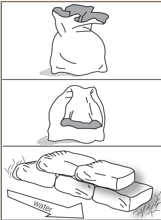
Figure C41. Sandbags are basically for low-flow protection of up to 0.6 meter (2 feet). Protection from higher flows requires a more permanent type of structure. It should be noted that sandbags will not seal out water.
