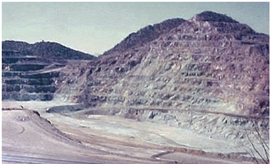
Figure C28. Schematic and photograph of rock benches. (Schematic from Reference 11, photograph of a mine in Tucson, Arizona, USA, by Steve Dutch, University of Wisconsin, USA.)
