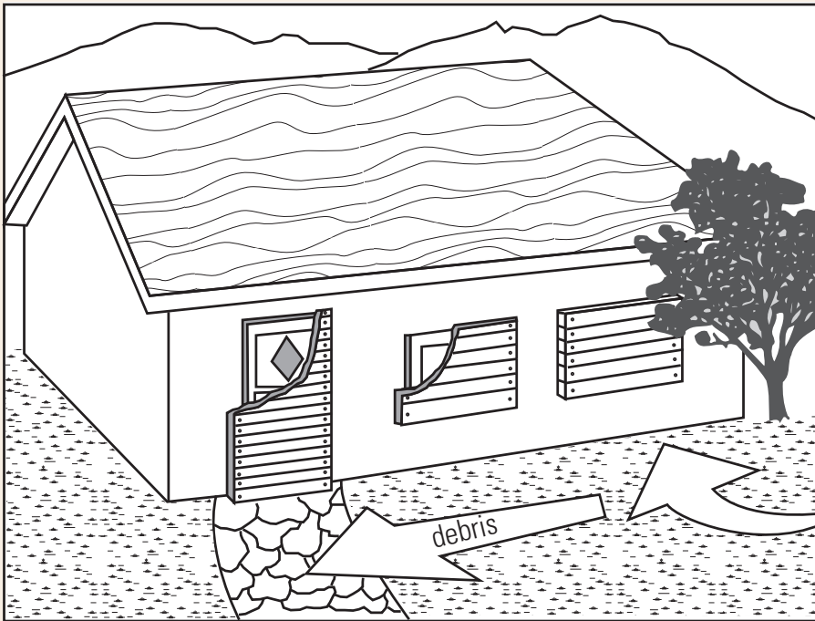
Figure C48. Nailing up plywood or lumber for window and door protection.
