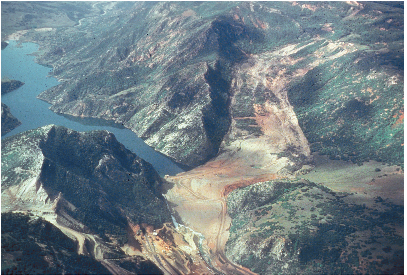
Figure C53. The Thistle landslide in Utah, USA, 1983. This landslide dammed a river, which formed a lake (called “Thistle Lake”) behind the dam, flooding the town of Thistle. (Photograph by Robert L. Schuster, U.S. Geological Survey.)
