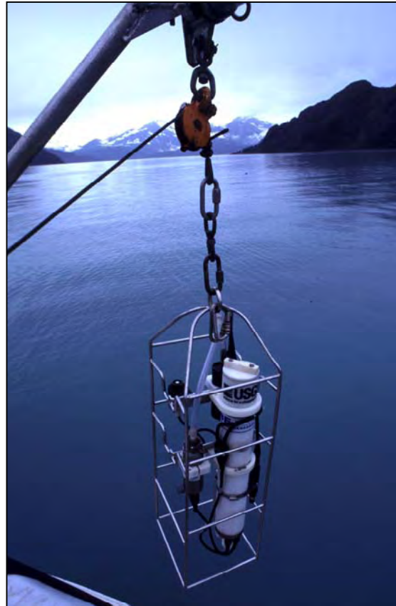
Figure 3. CTD apparatus ready for deployment on the RV David Grey .
