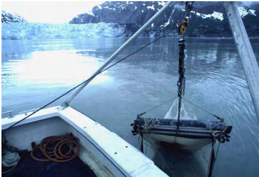
Figure 7. Deploying the Tucker Trawl at Station 21 (Margerie Glacier). Note tripping mechanism holding chains connected to net frames at top of net.
