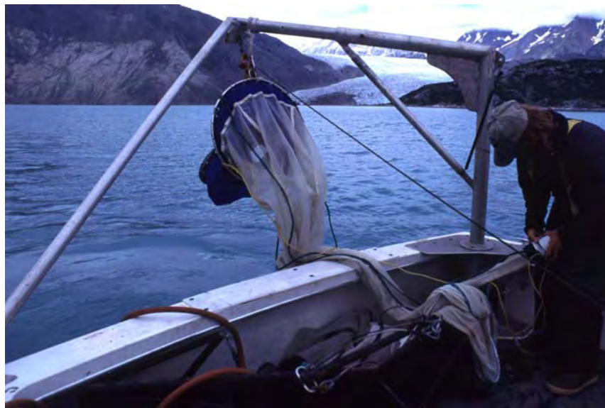
Figure 5. Preparing the vertical-haul zooplankton net for deployment at Station 18 in upper Muir Inlet.
