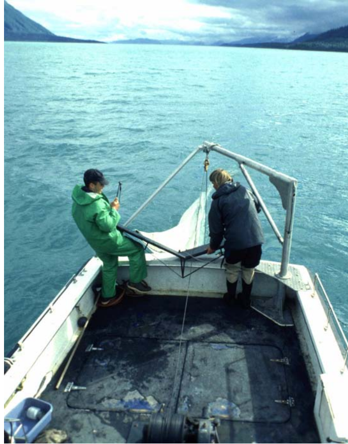
Figure 10 Deploying the Isaacs-Kidd mid-water trawl. Note the 'V' shaped depressor bar to which the net is attached.
