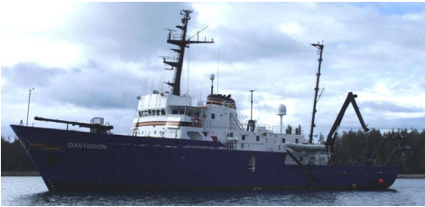
The survey vessel R/V Davidson, with a hull-mounted multibeam mapping system used to image almost half of Glacier Bay's waters deeper than 30 meters. The vessel also has an oceanographic laboratory that was used to obtain continuous measurements of phytoplankton density throughout the June, 2001 research cruise (figure to the right).
