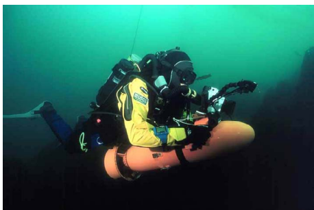
Diver conducting ground-truthing surveys with a diver propulsion vehicle, a digital video camera, and a mixed-gas rebreather. The diver is linked by communications and a transponder to a real-time data collection system in the support vessel. Photo by Jeff Mondragon.
