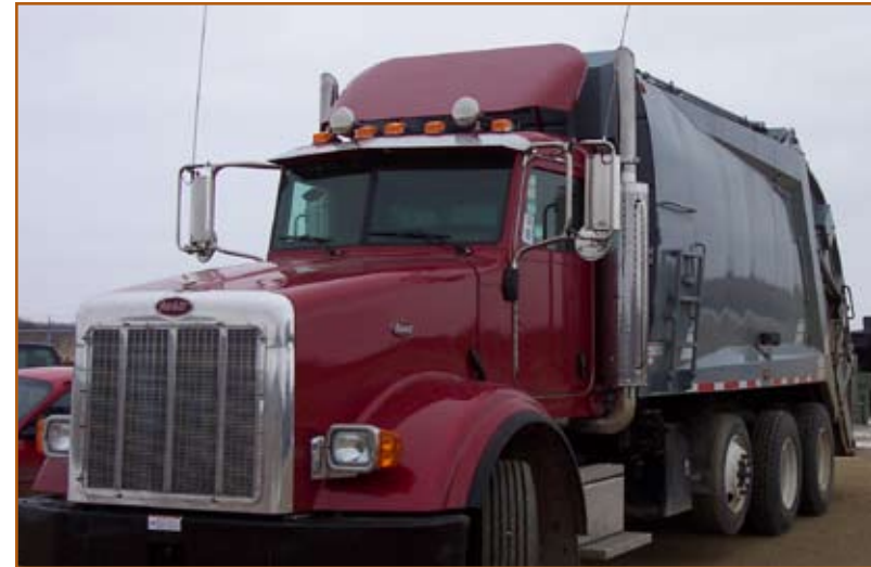
Figure 24: Twenty-five cubic yard, rear load compactor truck purchased for Spirit Lake Tribe Solid Waste Program.
