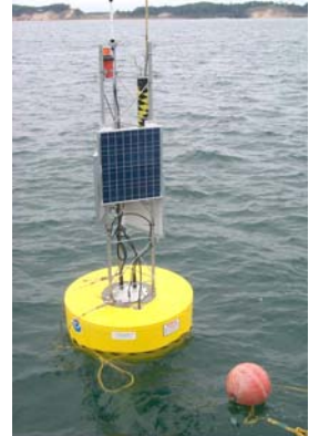
Portable Real-time Coastal Observation Network (ReCON) buoy. (photo: NOAA)
