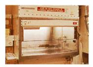
**Part 2** Alternatively, a Class 11, Type A cabinet can be equipped with a canopy or thimble unit which exhausts to the outdoors. For detailed information about the design, capabilities and limitations of various types of biological safety cabinets, refer to the National Sanitation Foundation Standard 49 *National Science Foundation. Standard 49 for Class 11 (Laminar Flow) Biohazard Cabinetry.*
