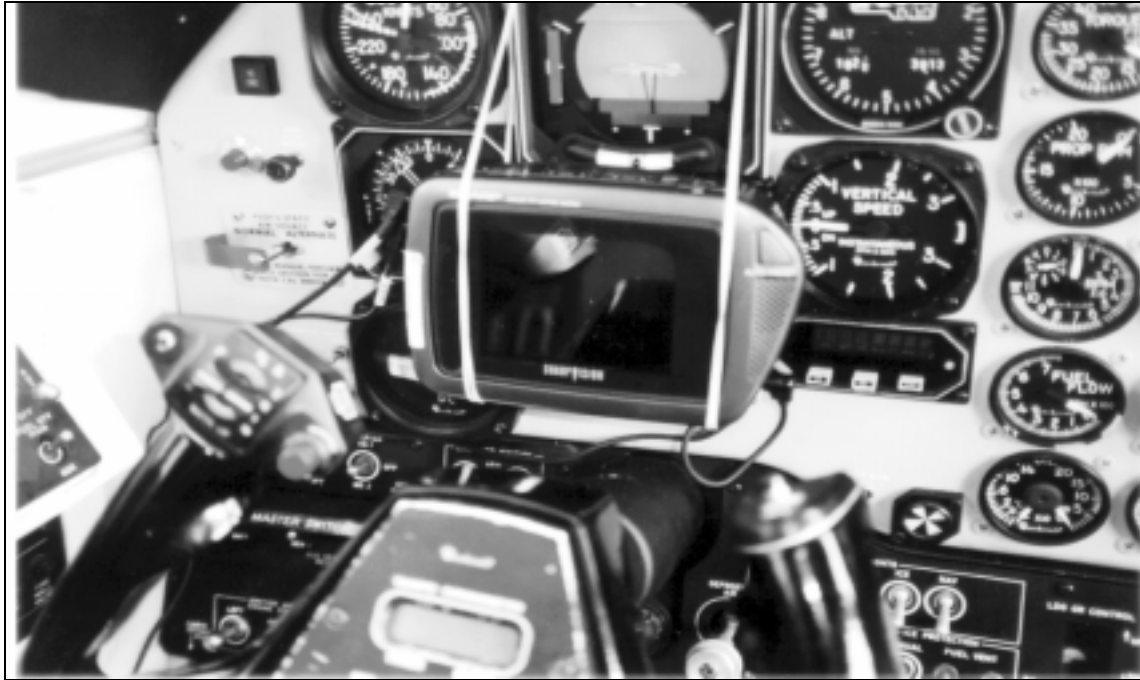
Figure 2-8. Attitude Display Temporarily Installed in the Cockpit of the Beechcraft 1900C
