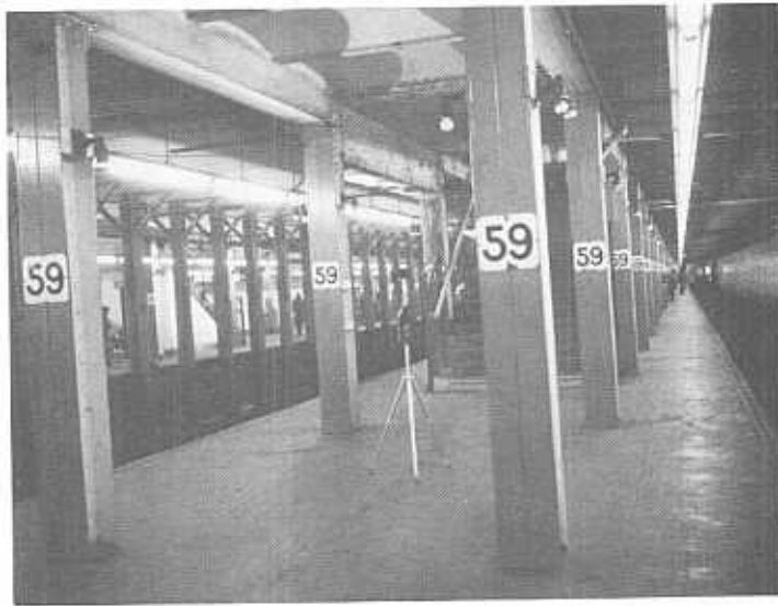
Figure F-4: Two Views of Microphone Located on Passenger Platform in 59th. St. Subway Station, NY City Transit System.
