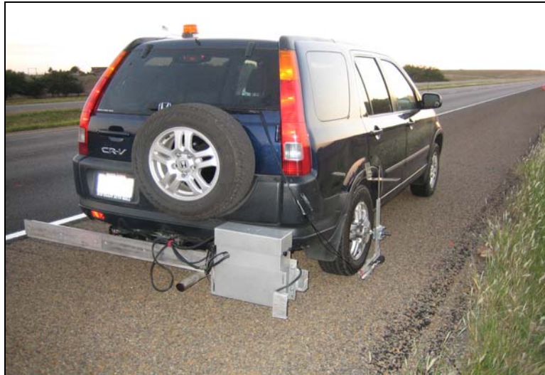
Figure 30. Laser profiler mounted behind the test vehicle.
