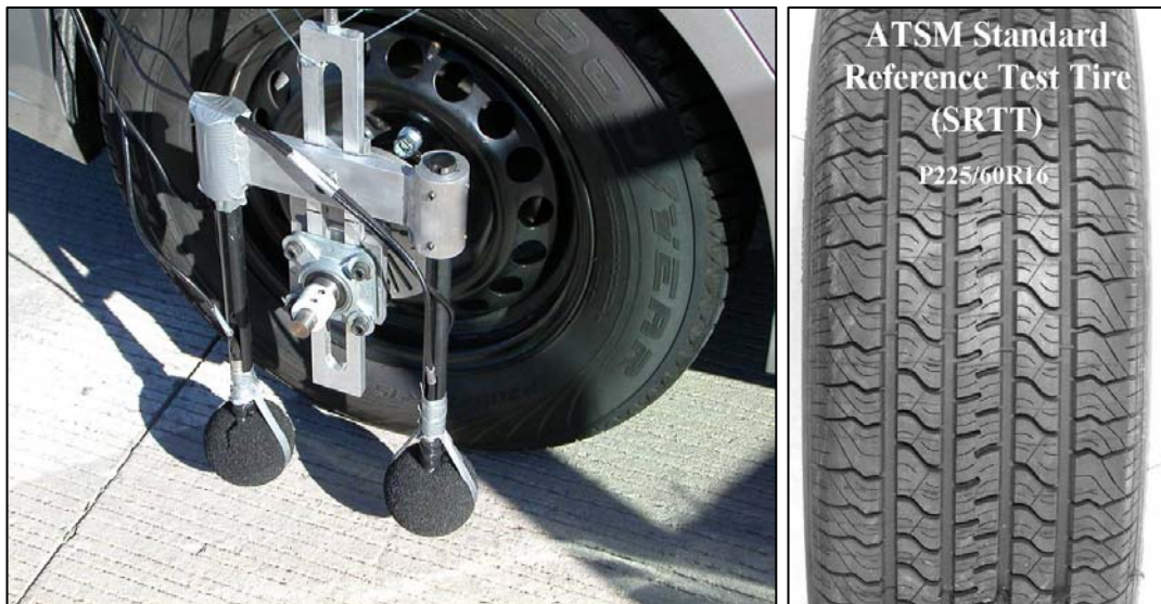
Figure 28. OBSI dual probe system and the SRTT.
