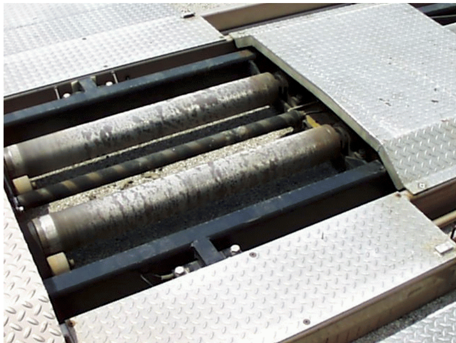
Figure A19. Hicklin Engineering, Inc. (HEI) portable roller dynamometer: overview (top) showing the ramps, the rollers and the operating console. The bottom picture details the two drive rollers and the smaller speed and vehicle position sensing roller on one side of the tester.
