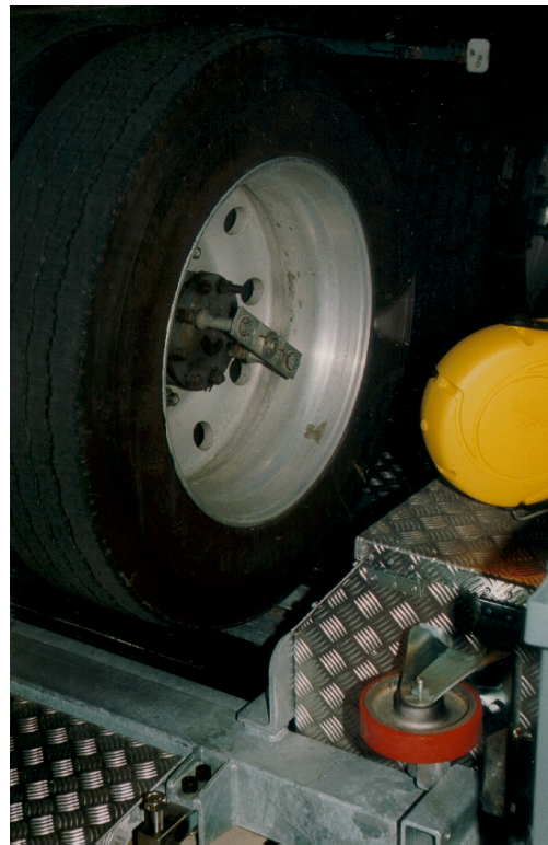
Figure A15. Radlinski and Associates, Inc. (RAI)/BM portable roller dynamometer: side view while testing the 3-S2 steer axle (top) and detail (bottom) showing the positioning of the wheel on the right side roller.
