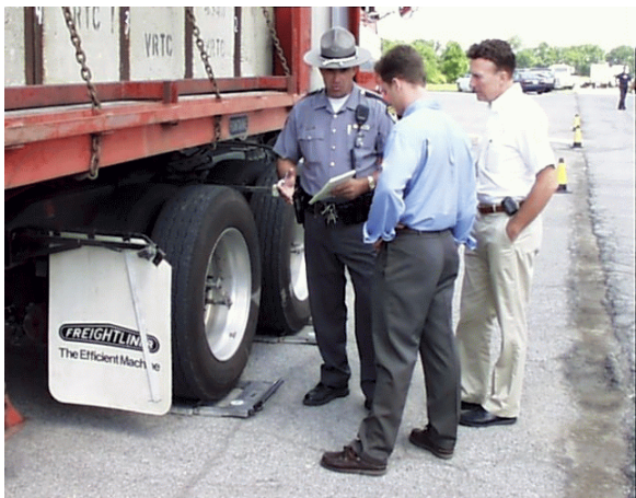
Figure A3. Axle and vehicle weights were measured using in-ground and portable certified scales. The use of portable scales increases accuracy as the vehicle is level with respect to the ground and all wheels are weighted simultaneously.
