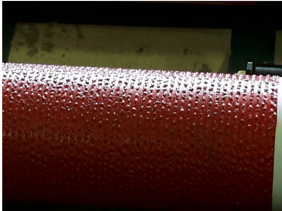
Figure A18. Vehicle Inspection Systems (VIS) portable roller dynamometer showing the two drive rollers and the smaller speed sensing and vehicle position roller (top) and detail of the test surface (bottom).
