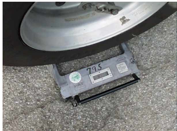
Figure A3. Axle and vehicle weights were measured using in-ground and portable certified scales. The use of portable scales increases accuracy as the vehicle is level with respect to the ground and all wheels are weighted simultaneously.
