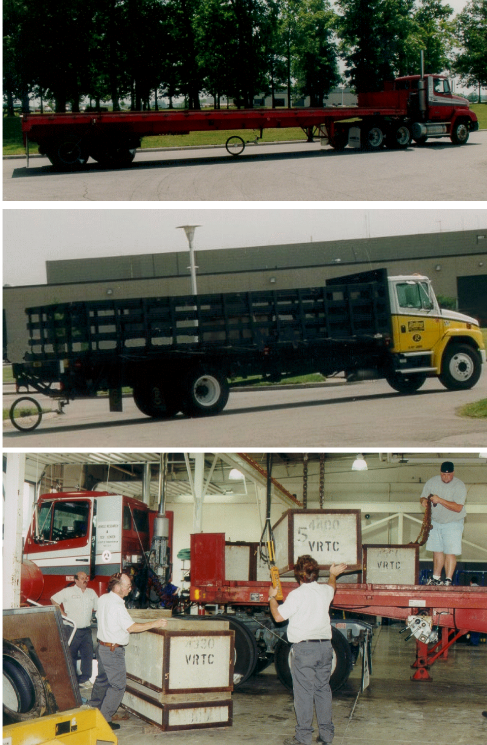
Figure A2. Test vehicles: 3-S2 tractor trailer combination (top) and 2-axle straight truck (middle), equipped with a fifth wheel. Loading and unloading with concrete blocks was facilitated by the use of flatbed trailers (bottom).
