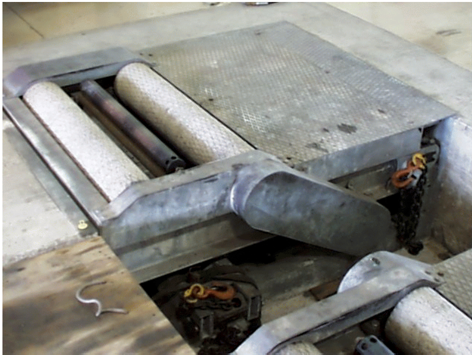
Figure A11. VRTC/BM in-ground roller dynamometer: overview (top) and detail (bottom) showing the sets of two driving rollers as well as the third smaller roller which monitors the wheel speed and the presence of a vehicle axle.
