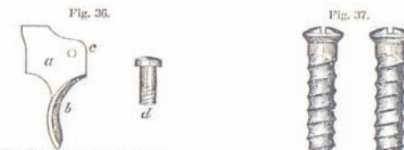
Fig. 36. Trigger, half size. a , blade; b , finger-piece; c , hole for screw; d , screw, full size.
