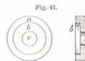
Fig. 41. Side-screw washer, full size. a , body; b , countersink; c , hole for screw.
