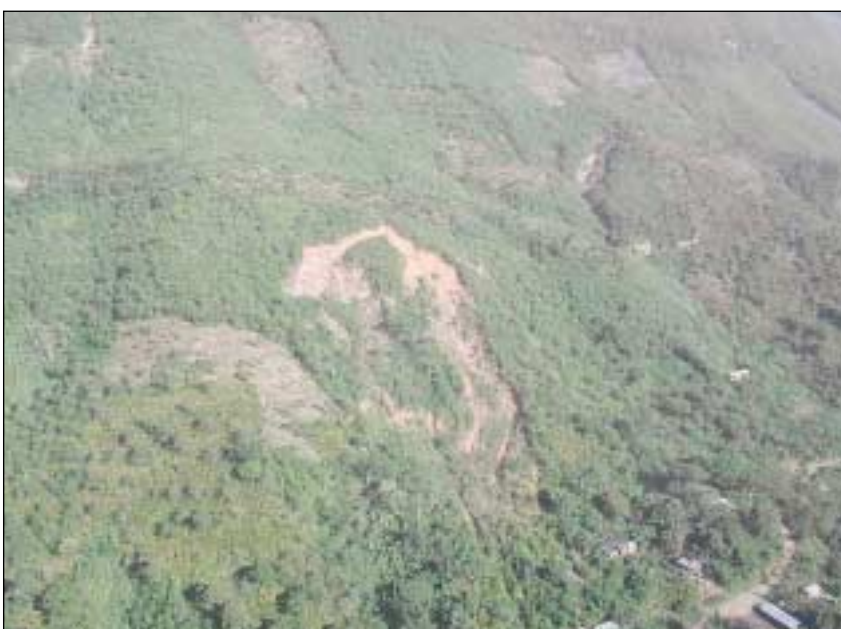
Figure 10. Landslide typical of the area northwest of Senahú; landslide is about 70 m wide and 400 m wide. View is to the north. UTM coordinates 193850 E, 1711100 N. Photo taken January 6, 2001.
