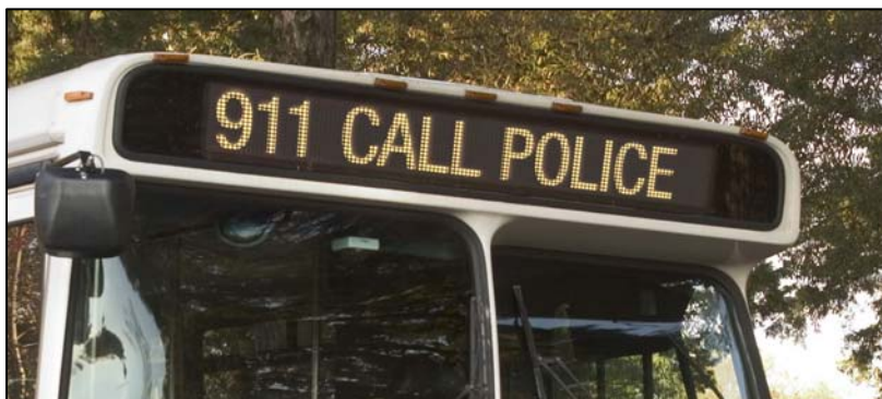
FIGURE 3.14 – Using Destination Signage Systems for Security Purposes
