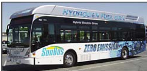
SunLine fuel cell hybrid bus. Photo courtesy of SunLine.
