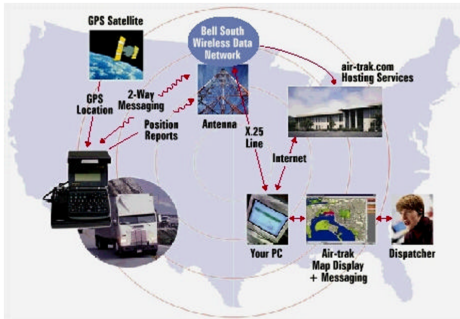
Figure 2-5. Air-Trak AVL Wireless GPS System Overview
