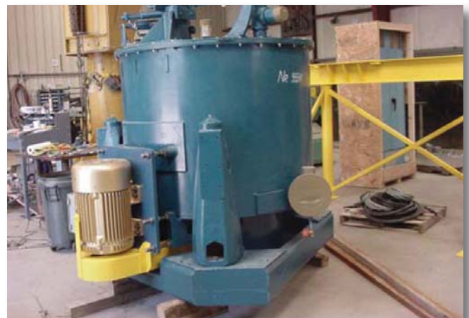
The Triton TS-5000 Separator is one of three solids separation technologies evaluated by the Water Quality Protection Center for the treatment of flushed swine waste.
