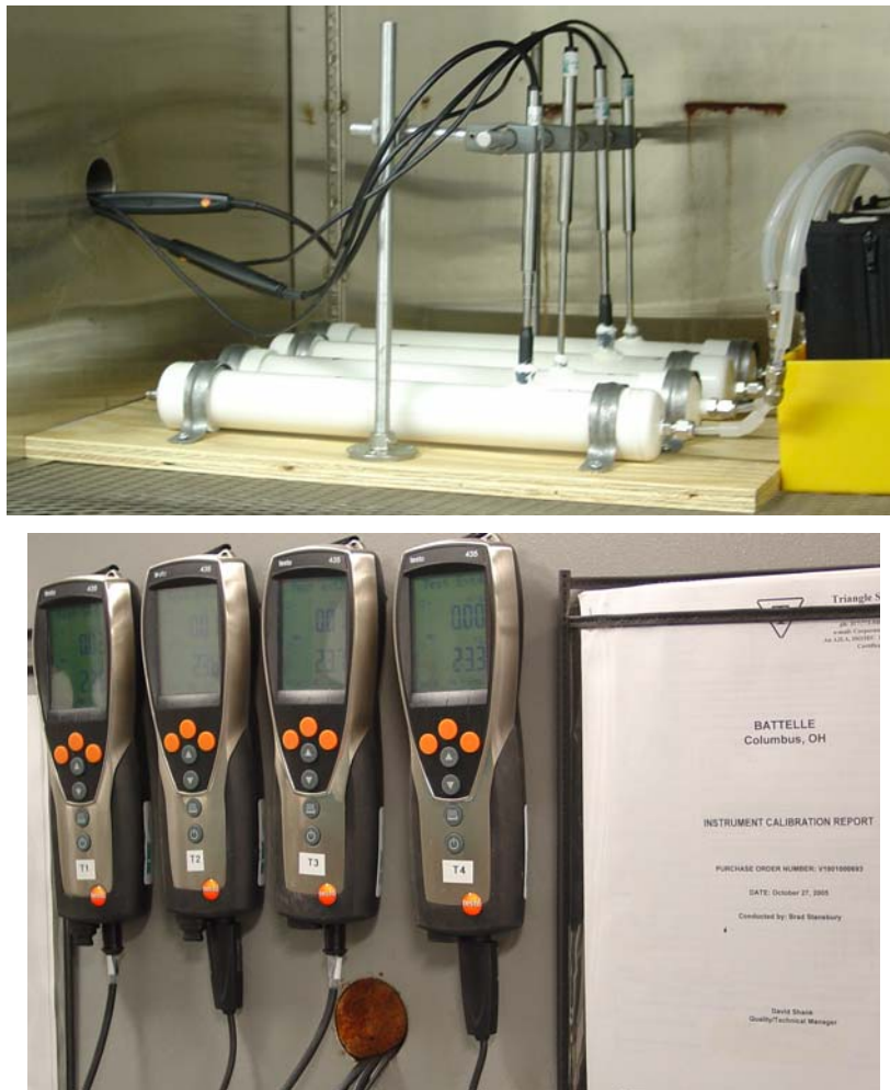
Figure 3-3. Leland Legacy ® Pumps (4) Connected to Flow Cells Equipped with Hot Wire Anemometers in a Constant Temperature and Humidity Chamber (top) for the Extreme Temperature (40°C) and Moderate/High Humidity (60/90%) Tests. Data Logging Velocity Meters Used to Monitor the Pumps' Flow Performance Were Located Outside the Chamber (bottom).
