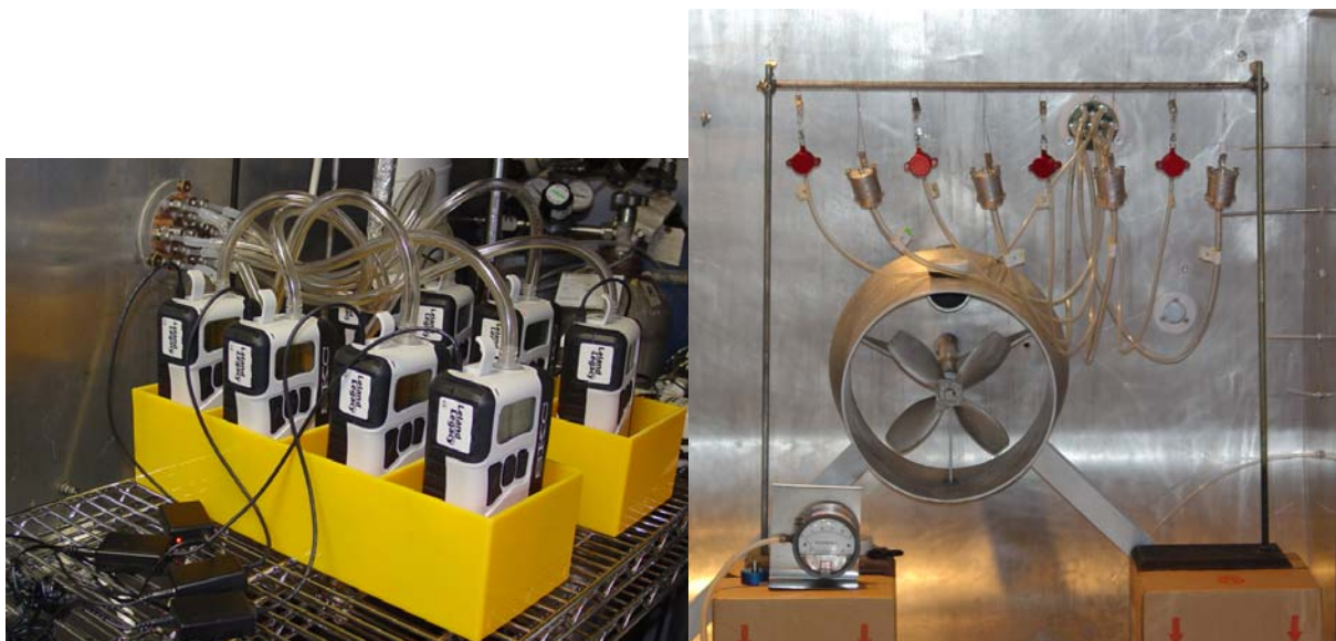
Figure 3-8. The Leland Legacy ® Pumps Were Placed Outside the Large Environmental Chamber (left), and Were Connected via Feedthroughs to the Test Sioutas PCIS and Reference PEM Samplers Inside the Chamber (right).
