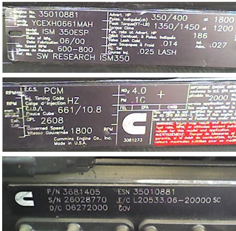
Figure 2. Identification labels for 2000 Cummins ISM350 engine and its electronic control module.
